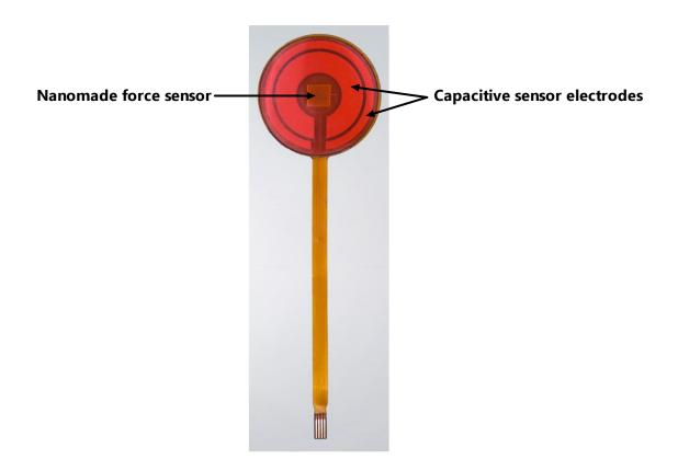
This sensor is composed of only one copper layer on polyimide substrate. Both capacitive and force sensors electrodes are designed on this unique layer.
