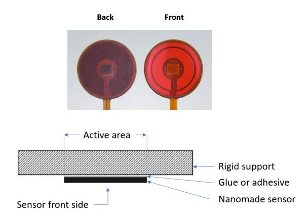
The higher the deformation transmitted to the sensor, the higher the variations of the sensor signal output. To glue the sensors to the surface adapted to your needs it is strongly recommended to use a rigid glue. The following three glues have been tested and are valid for your tests, the references are given in the table below.
